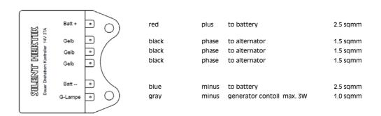
The minus plug which connects the alternator controller and the battery is obligatory! If there is a loose connection between alternator and battery, it will blow a fuse and lead to total failure. The crimp-connectors MUST be handled with quality pliers.
