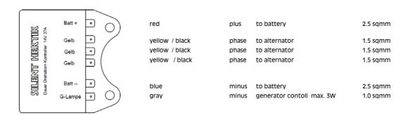
The minus plug which connects the alternator controller and the battery is obligatory! If there is a loose connection between alternator and battery, it will blow a fuse and lead to total failure. The crimp-connectors MUST be handled with quality pliers.
