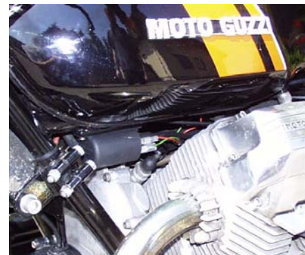
coil assembly on the frame for cooling
