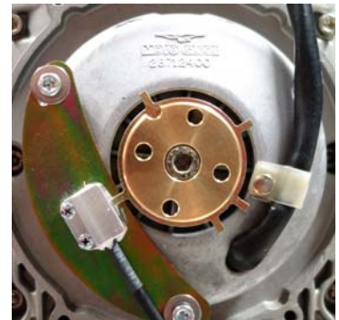
static position of the trigger system on the Saprisa alternator. The Rotor should be in the middle of aluminium housing with a 0,6-0,8mm gap
