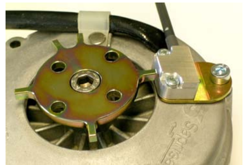
static position of the trigger system on the Saprisa alternator. Fix the sensor with a M3 screw. The Rotor should be in the middle of aluminium housing
