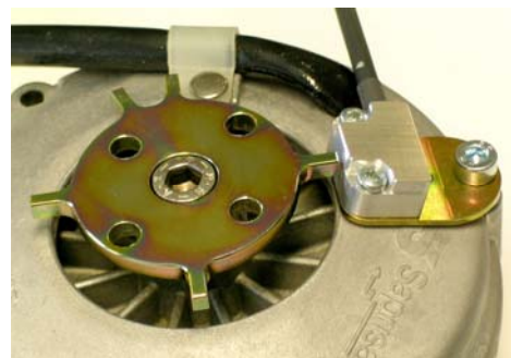
static position of the trigger system on the Saprisa alternator. Fix the sensor with a M3 screw. The Rotor should be in the middle of aluminium housing
