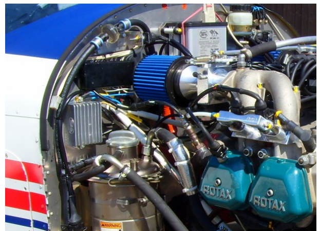
Installation in the front with good cooling by airflow and max. 70cm cables to the battery
