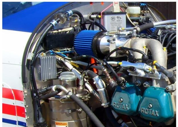
Installation in the front with good cooling by airflow and max. 50cm cable to the battery
