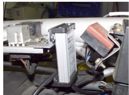
The distance from the box to coils should be min. 10cm
