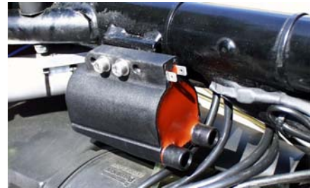
PowerCoil on the /5 frame The ignition-box can be mounted on the other side
