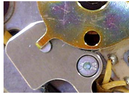
inductive pickup on the Bosch alternator
