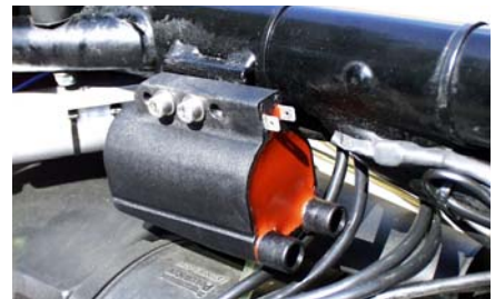
PowerCoil on the 1/5 frame The ignition-box can be mounted on the other side
